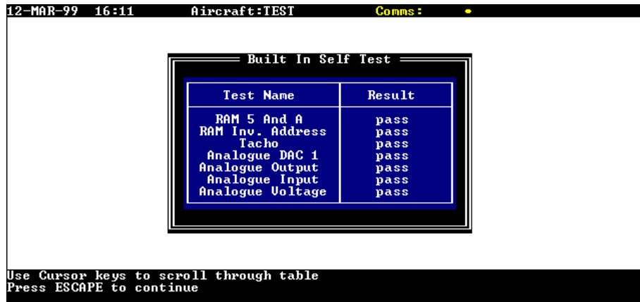
Figure 3.31 – 'Built In Self Test' results screen
