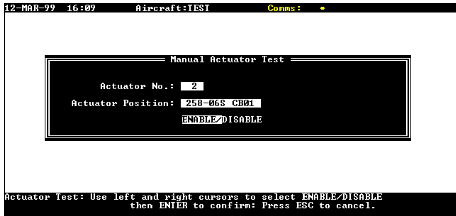
Figure 3.20 – 'Manual Actuator Test' screen.
