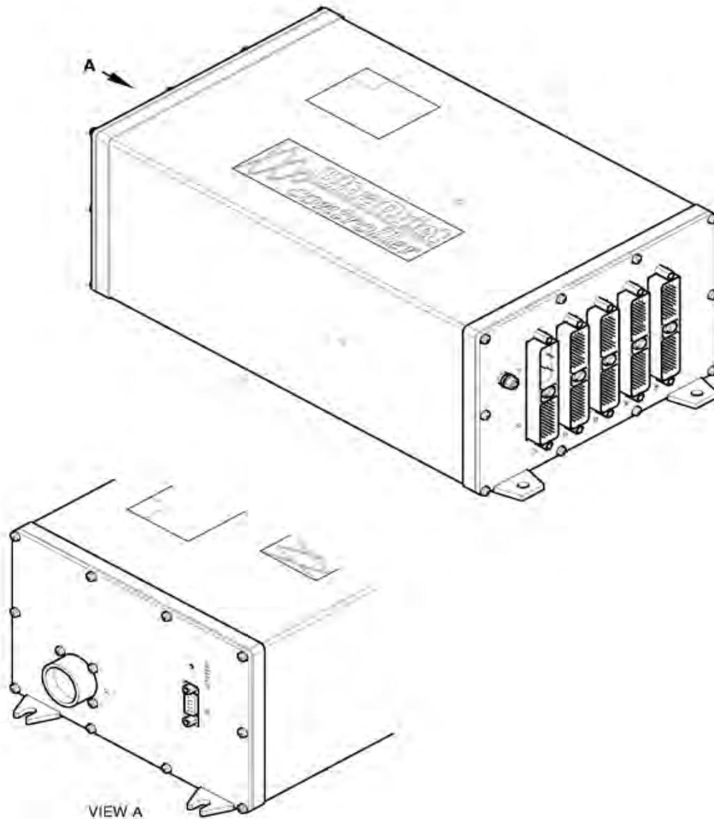
**Figure 1-1 Active Noise Control Unit (ANCU)**
