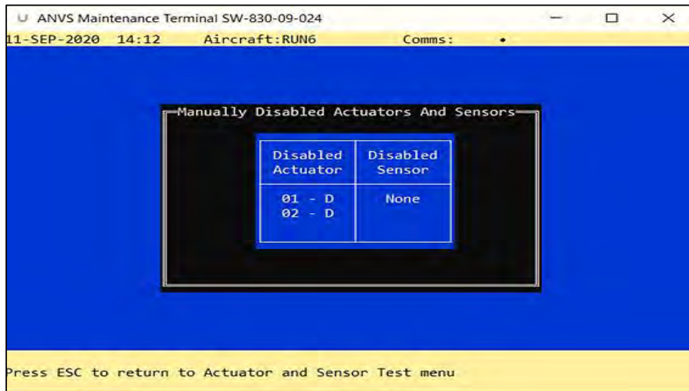
Figure 4-12 Manually Disable Actuators and Sensors
