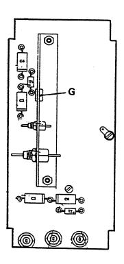
Figure 1 Power Supply/Filter Assembly - Grommet Positions
